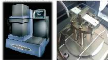
Figure 1. Views of a) DMA Q800 Dynamic Mechanical Analyzer and b) calcium phosphate sample mounted on the three point bending supports of the DMA device.
